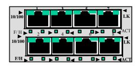
into an RJ-45 port and the Link (LK) indicator for that port must be ON (indicating there is a powered-up device at the other end of the cable) in order for a LK LED to provide valid indications of operating conditions on that port.
